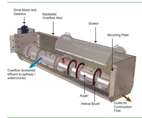
Flows enter the chamber causing water levels to rise, initiating the rotation of the helical brush mechanism on the influent side of the screen, and begins to flow through the Heliscreen®'s semicylindrical stainless steel perforated screen (red arrow).
