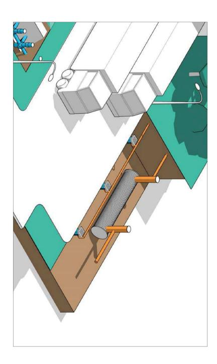
When planning and installing percolation systems, effective rainwater pre-treatment, even beyond natural cleaning mechanisms like soil passages, is becoming increasingly important.
