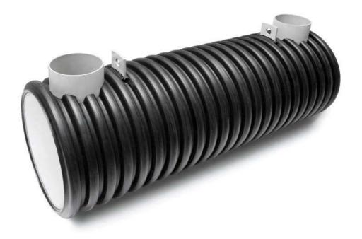
The RAUSIKKO SediClean facilitates effective retention of the finest particles. It uses the force of gravity to separate contaminants from less-contaminated water. As the sedimentation volume steadily accumulates, the fine particles begin to settle.
